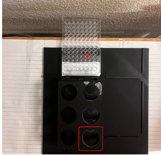
Figure 3: Top view of the experimental setup. The upper red square marks the tube starting position, and the larger lower red square marks the goal position for the tube.
